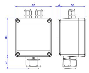
The instrument is based on fully calibrated, linearised and temperature compensated semiconducting metal-oxide gas sensor with high repeatability, stability and long lifetime. The sensor exhibits high sensitivity to ammonia.
